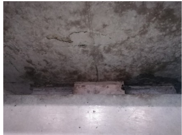
(a) Load-drift relationship (b) Punching shear failure
