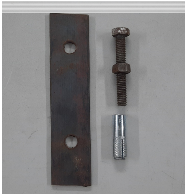
Figure A.2.57: Flat bar, rawl bolt and nut bolt details to connect existing brick and beam with wire mesh
