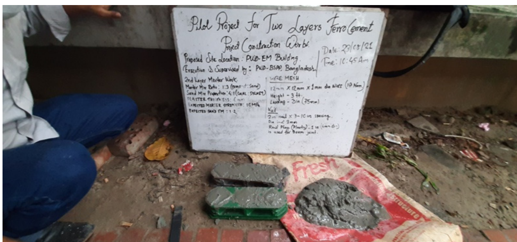
Figure A.2.64: Cube preparation for checking the strength of prepared mortar
