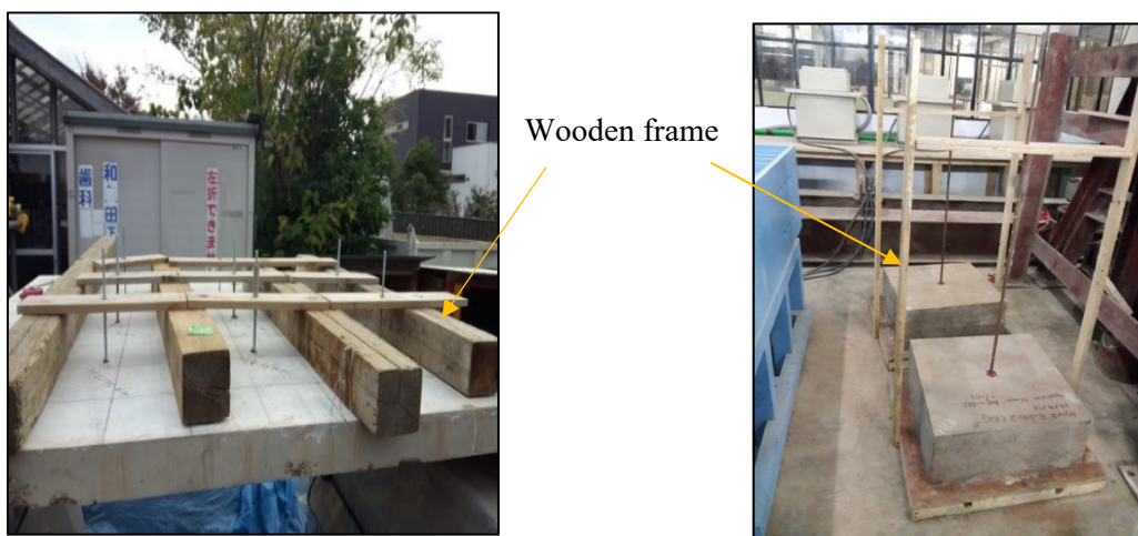
Figure C.4.4 Temporary wooden supports of anchor and rebar (from left)
