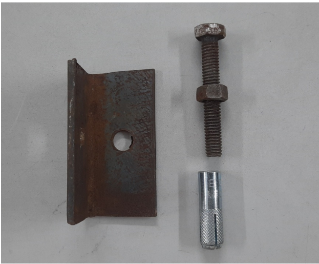
Figure A.2.56: Angle, rawl bolt and nut bolt details to connect existing brick and column with wire mesh (where the thickness is adequate)
