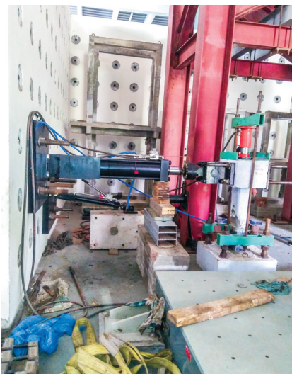
Column Test by Actuator
