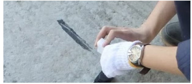
Scratching the concrete surface
