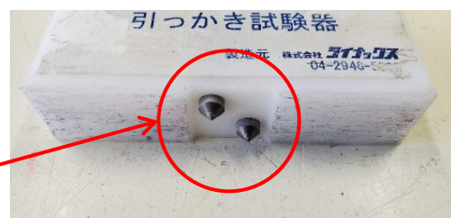
Pins to make grooves by scratching the concrete surface
