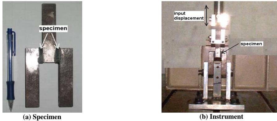
Figure 2. Specimen and instrument of simple shear experiment
