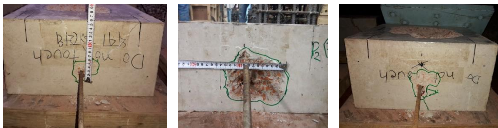
Fig. 12 – Failure modes from shear test of post-installed bonded anchors (S1, S2, S4 from left)
