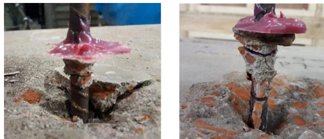
Fig. 9 – Bond failure of steel/adhesive interface and adhesive/concrete interface (from left)
