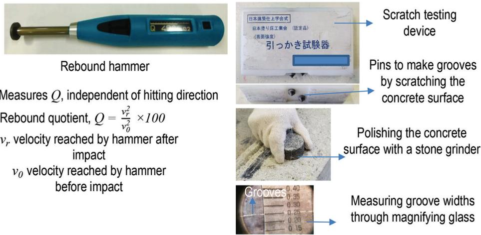
Fig. 1—Low-energy nondestructive test devices.
