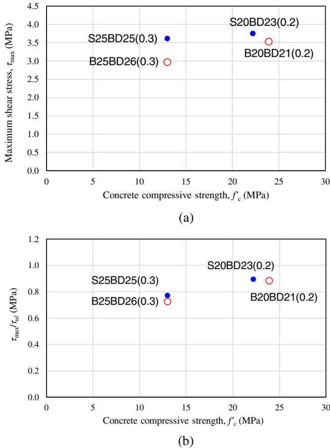
FIGURE 6 Assessment of results obtained from experiments. (a) Normalized tested shear strength (shear stress)  $\tau_{max}$ . (b) Accuracy of the shear strength estimation.
