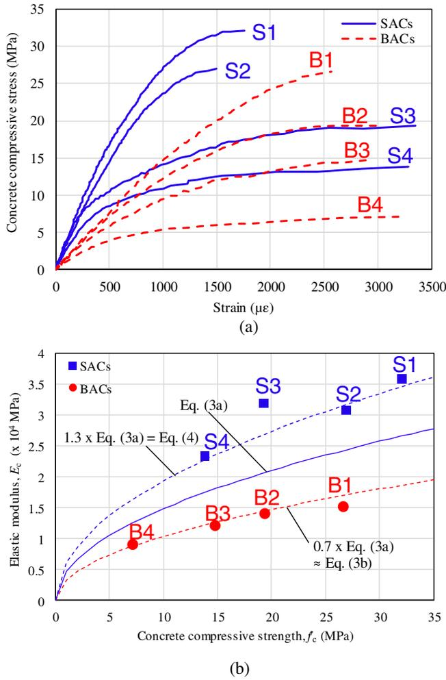
**FIGURE 3** Stress–strain responses and elastic modulus seen for grades of brick aggregate concrete (BAC) and stone aggregate concrete (SAC) in experiments. (a) Stress–strain responses. (b) Variation of  $E_c$  with  $f'_c$ .
