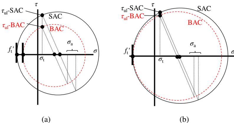
FIGURE 7 Conceptual diagrams of Mohr's circle at the computed ultimate shear strength considering the difference in materials. (a) low-strength ( $f'_c \approx 13$  MPa) specimens. (b) mid-strength ( $f'_c \approx 23$  MPa) specimens.
