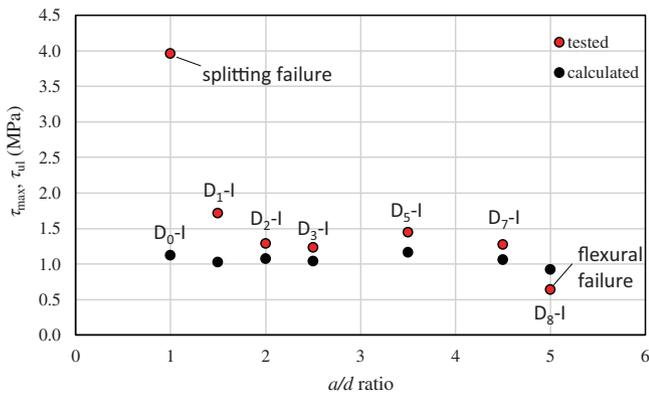
FIGURE 9 Comparison between tested strength ( $\tau_{max}$ ) and estimated strength ( $\tau_{ul}$ ) for the specimens and test results presented in Akhtaruzzaman and Hasnat.<sup>18</sup>
