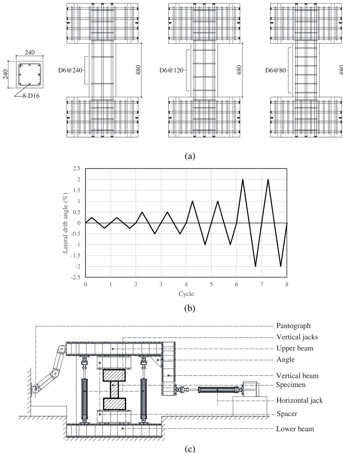
**FIGURE 4** Testing of specimens from brick aggregate concrete (BAC) and stone aggregate concrete (SAC). (d–g) Typical failure patterns in tested specimens. (a) Specimen geometry and rebar details. (b) Applied loading history on each of the specimens. (c) Specimen in the test setup as seen in the elevation view. (d) B20BD21(0.2). (e) S20BD23(0.2). (f) B10BD26(0.3). (g) S10BD25(0.3).
