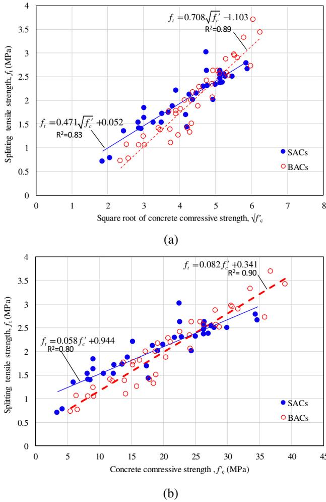
FIGURE 2 Relationships between compressive strength and splitting tensile strength observed from experiments. (a) Relation between  $f_t$  and  $\sqrt{f'_c}$ . (b) Relation between  $f_t$  and  $f'_c$ .
