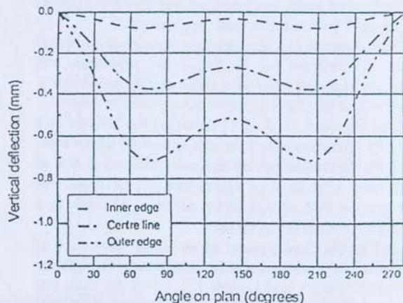
Figure 4: Vertical displacements (Stair-II)
