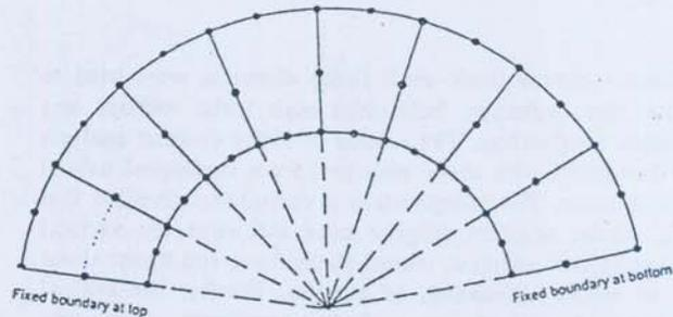
Figure 2: FE mesh used in the investigation
