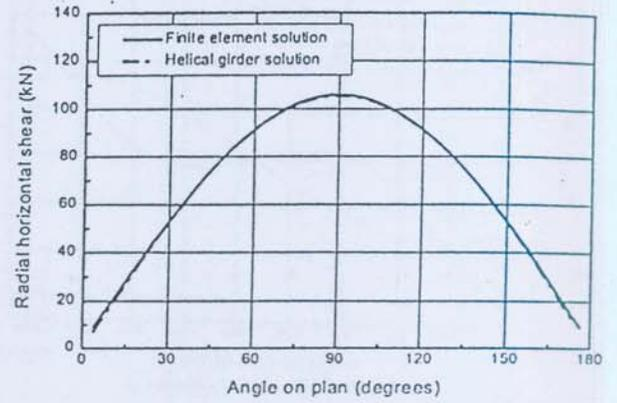
Figure 10: Radial horizontal shear (Stair-I)
