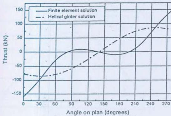
Figure 14: Thrust (Stair-II)
