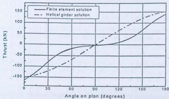
Figure 8: Thrust (Stair-I)
