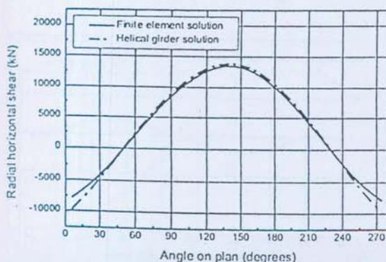
Figure 16: Radial horizontal shear (Stair-II)
