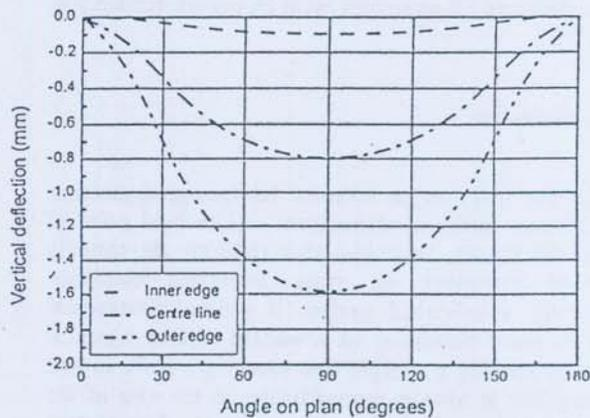
Figure 3: Vertical displacements (Stair-I)
