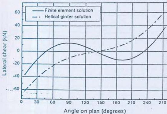
Figure 15: Lateral shear (Stair-II)
